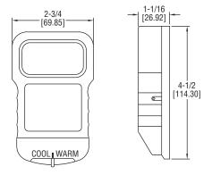
The Series WTP-W Wireless Wall Mount Temperature Sensors allows flexibility in office buildings with cubicles or in hotel rooms. Without any wires to limit the location of the sensor, it can be moved quickly without any interruption in temperature measurement. Optional temperature set point and manual override features allow users to adjust temperatures to make the ambient conditions more comfortable.
