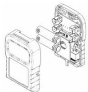
Figure 2: Polarity of Battery Installation
