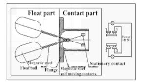
UOK(S)-100 float level switch structure schematic diagram
