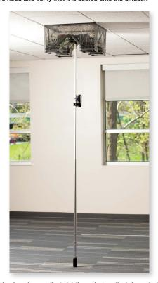
Once the hood is placed correctly, twist the pole to adjust the pole length so that it reaches the floor supporting the hood itself. If the hood is not securely in place, then re-adjust the pole length until it is free standing.
