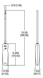
The Series AP3 Wireless Thermo-Anemometer Probe measures air velocity, air flow, and temperature when combined with the UHH4 or newer universal handheld device, or your own mobile device. In order to prevent damage to the sensing element, the probe has a protective sleeve that slides over the sensor when it is not in use. Markings on the probe allow users to know the insertion depth to obtain better accuracy when traversing the duct.
