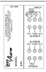
Power for SC1290 is 85 to 265 Vdc/Vac 50 to 400 Hz. Power for SCL1290 is 12 to 24 Vdc/Vac 50 to 400 Hz.
