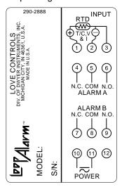
For SC1090, power is 85 to 265 Vdc/Vac 50 to 400 Hz. For SCL1090 power is 12 to 24 Vdc/Vac 50 to 400 Hz. ±20%.
