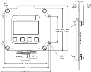
**Wall Mount.** To mount an RTI2 indicator to the wall, hold the unit in the desired position, mark the holes in the mounting feet, drill and mount with screws. A meter-mounted indicator can be converted to a wall mount using an adapter mounting kit. Contact distributor for information.
