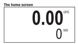
The HOME Screen, shown above, is the normal screen which displays TOTAL flow volume and flow RATE. The Four buttons below the LCD display are used to access menu screens for viewing and changing setup parameters.
