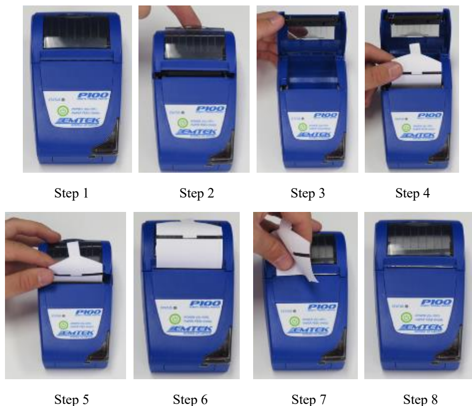
Fig 7.4.1 Loading Paper, or Label Roll in Thermal Printer
