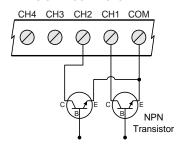
Figure 10. Open Collector NPN Transistor Inputs
