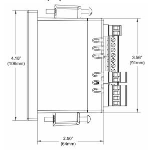
Figure 2. Case Dimensions - Side View
