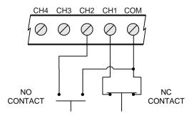
Figure 9. NO/NC Contact Inputs
