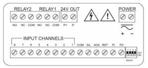
Figure 5. Connector Labeling for AN28-1
