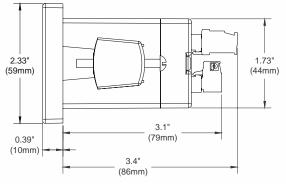
Figure 3. Case Dimensions - Top View
