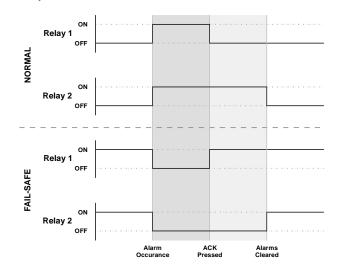
**Relay On:** Relay is energized **Relay Off:** Relay is de-energized.
