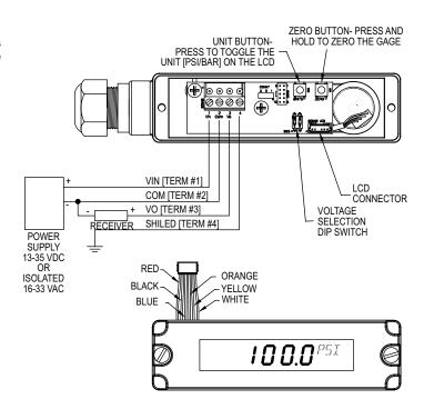
Figure 6: Voltage output with optional LCD
