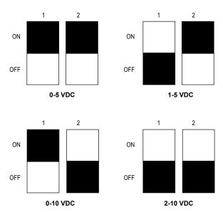
Figure 4: Voltage output DIP switch selection
