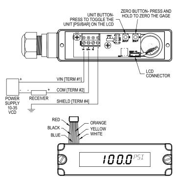
Figure 2: Current output with optional LCD
