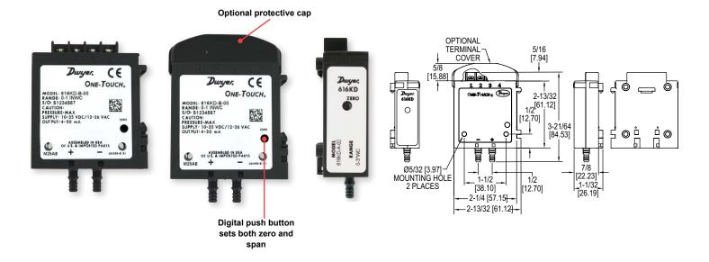
The Series 616KD One-Touch® Differential Pressure Transmitter senses the pressure of air and compatible gases and sends a standard 4-20 mA or optional voltage output signal. A wide range of models are available factory calibrated to specific ranges. A single push button properly adjusts both zero and span. New enclosure enables the 616KD-A/B to be mounted on a 35 mm DIN rail either via its side or back DIN rail clips.
