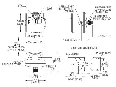
One of our most popular differential pressure switches is now available with a DPDT switch. The 1831 combines small size with 4% set point repeatability. Absolutely no power is required to operate the DPDT switch. Set point adjustment on the switch is easily accessible for modifying the set point. A mounting bracket is included for simplified installation.
