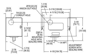
Series AP Diaphragm Operated Pressure Switches are reliable, convenient, compact, low-cost switches for instrument air or other low-pressure applications. Visible set point and external adjustment add convenience. Used on air, noncorrosive gas or liquid service compatible with wetted parts. These switches are available with optional weather-proof and explosion-proof housings.
