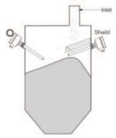
Figure 5 - Side Mounting Installation
