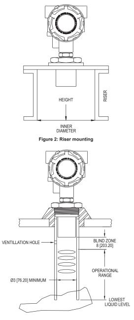
Figure 3: Stand pipe mounting
