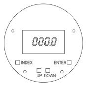
Figure 5: Display and programming buttons
