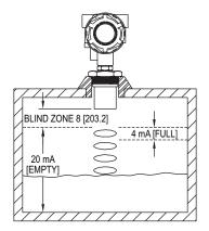
Figure 7: Reverse output operation
