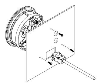
Figure 3: Surface assembly with rear pressure connections
