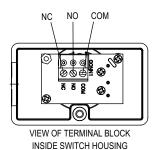
Figure 2: Wiring Diagram
