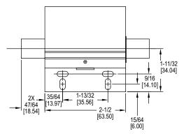
Figure 2: Mounting Hole Dimensions
