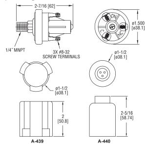
Series A6 Durable Pressure Switches have been specifically designed to stand up to extended duty applications. These switches are constructed with a polyimide film diaphragm and are compatible with a variety of fluids. For ease of installation, the switches come with a 1/4" male NPT process connection and can be mounted in any orientation. The Series A6 pressure switches are compact and have great setpoint integrity, and feature simple, easy set-point field adjustment.
