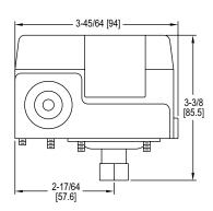
The Series CXA Water Pump Pressure Switch has been proven reliable for controlling automatic water systems. These switches are very popular for use on water well pumps and pumping systems. The set point and deadband are both easily adjustable via screws inside the cover. For ease of installation, the switches come with a 1/4" female NPT process connection and can be mounted in any orientation. The series CXA's simple design makes it a great switch for an installer at any skill level.
