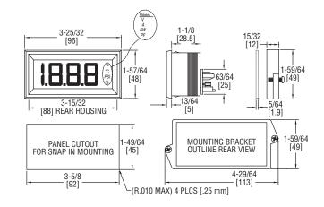
Series DPMA-4 Adjustable LCD Digital Panel Meter offers a 3-1/2 digit display for easy viewing in a standard 1/8 DIN package. Unit accepts 4 to 20 mA DC inputs with a wide bipolar span and zero adjustment. Standard features include field selectable engineering units and decimal point positions. Choose from red, amber, or green segments for easy viewing at a distance. A 24 VDC power supply is required for the operation of the backlight.
