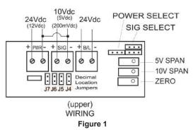
The unit is powered by a 12 or 24 VDC power supply and the screw terminals for wiring are located on the back of the adder board marked with + PWR - (see Figure 2). Move the power select jumper for the appropriate power supply value. The backlighting requires a 24 VDC power supply and should be connected to terminals identified with + B/L -.
