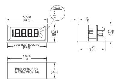
The Series DPML-5 LCD Digital Panel Meter is easy-to-read, even at a distance. The meter is designed with a large 4-1/2 digit LCD display with a choice of red, amber or green segments. The meter features adjustable zero and span, user selectable decimal point position, and selectable 12 VDC or 24 VDC power supply. The backlight requires a 24 VDC power supply. Installation is quick with the snap-in bezel mounting.
