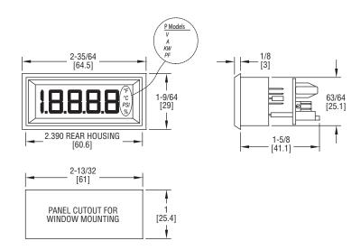
The Series DPML-4 LCD Digital Panel Meter offers a large 4-1/2 digit LCD display with a choice of red, amber or green segments for easy viewing at a distance. The meter accepts loop powered 4-20 mA DC input. Standard features include field engineering units and decimal point positions. A separate 24 VDC power supply is required for the operation of the back light.
