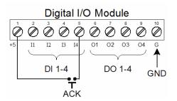
When the ACK button or the assigned digital input is closed, all relays programmed for manual reset are acknowledged.
