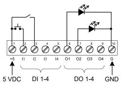
Figure 26. Digital I/O Module Connections
