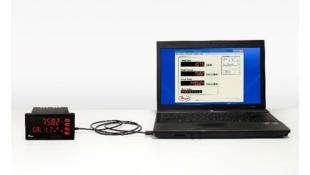
The meter can be powered from the Micro USB connection. When using the Micro USB connection, <u>**DO NOT**</u> apply AC or DC power to the meter.
