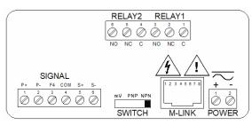
Figure 6. PPM-120 & PPM-220 Connectors Label
