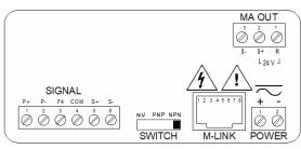
Figure 7. PPM-101 & PPM-201 Connectors Label
