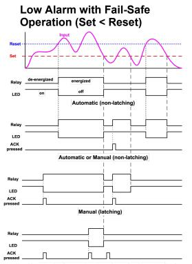
Manual only after passing above Reset (latching with clear) Note: Relay coil is energized in non-alarm condition. In case of power failure, relay will go to alarm state.
