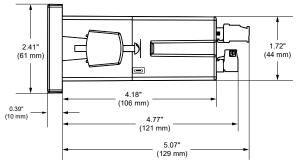
Figure 2: Meter Dimensions - Side View
