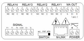
Figure 10. PPM-141 & PPM-241 Connectors Label
