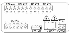
Figure 8. PPM-140 & PPM-240 Connectors Label
