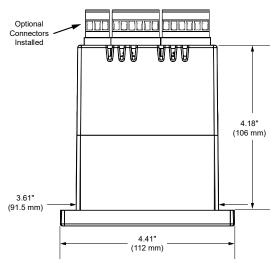
Figure 3: Meter Dimensions - Top View
