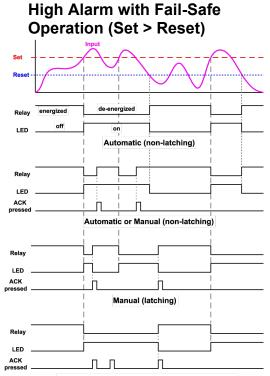
Manual only after passing below Reset (latching with clear) Note: Relay coil is energized in non-alarm condition. In case of power failure, relay will go to alarm state.
