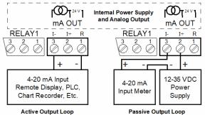
Figure 20. 4-20 mA Output Connections
