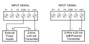
Figure 14. Transmitter Powered by External Supply or Self-Powered
