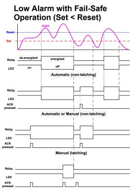
Manual only after passing above Reset (latching with clear) Note: Relay coil is energized in non-alarm condition. In case of power failure, relay will go to alarm state.
