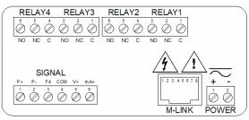
Figure 9. MPM-140 & MPM-240 Connectors Label
