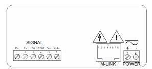
Figure 6. MPM-100 & MPM-200 Connectors Label
