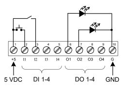
Figure 24. Digital I/O Module Connections
