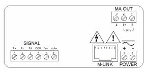
Figure 8. MPM-101 & MPM-201 Connectors Label
