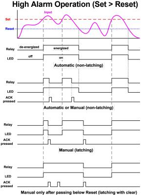
For Manual reset mode, ACK can be pressed anytime to turn "off" relay. To
