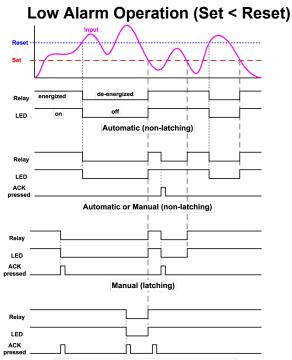
Manual only after passing above Reset (latching with clear)
