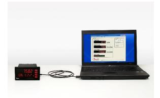
The meter can be powered from the Micro USB connection. When using the Micro USB connection, <u>**DO NOT**</u> apply AC or DC power to the meter.
