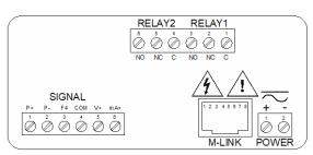
Figure 7. MPM-120 & MPM-220 Connectors Label
