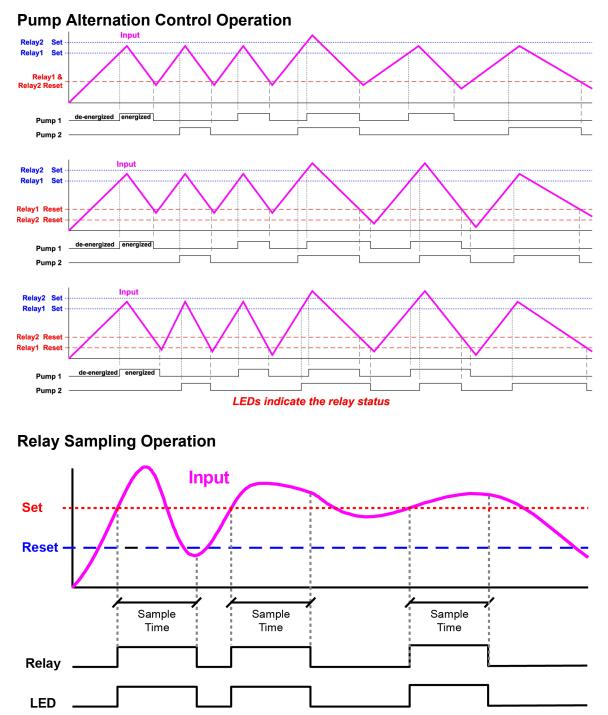
When the signal crosses the set point, the relay trips and the sample time starts. After the sample time has elapsed, the relay resets. The cycle repeats every time the set point is crossed, going up for high alarms and going down for low alarms.
