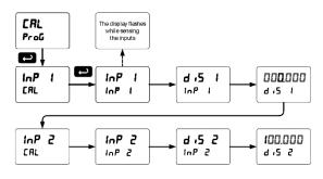
Warm up the meter for at least 15 minutes before performing calibration to ensure specified accuracy.
