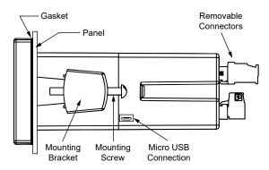
**<u>DO NOT</u>** apply AC or DC power to the meter when using the Micro USB connection.
