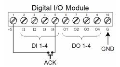
When the ACK button or the assigned digital input is closed, all relays programmed for manual reset are acknowledged.
