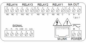
Figure 11. MPM-141 & MPM-241 Connectors Label
