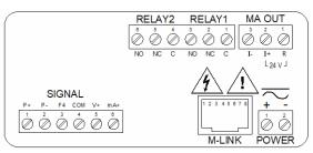
Figure 10. MPM-121 & MPM-221 Connectors Label
