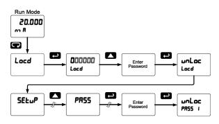
If the correct six-digit password is entered, the meter displays the message unloc (unlocked) and the protection is disabled until a new password is programmed.
