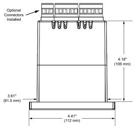
Figure 4. Meter Dimensions - Top View
