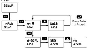
Set d-5[RL to no if only one scale is needed for the input.
