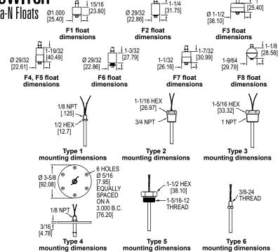
The Series F7-MM Miniature Multi-Station Level Switch provides a customized level switch to meet application requirements in a miniature size. Control up to five different level points across a maximum length of 48" (121 cm). Stems and mounting fixtures are available in 316 SS or brass.
