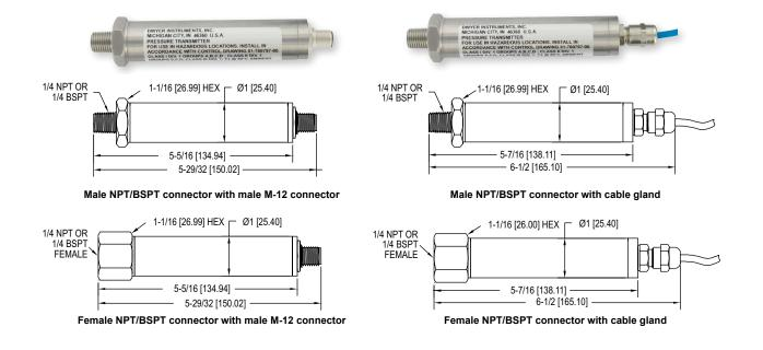
The Dwyer **Series IS626 Pressure Transducer** convert pressure into a standard 4-20 mA output signal. The Series IS626 can be used to accurately measure compatible gases and liquids. Series IS626 full scale accuracy is 0.25% (see specifications). Designed for industrial environments with a NEMA 4X (IP66) housing, this transmitter resists most effects of shock and vibration.
