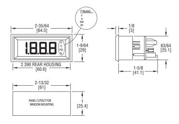
The Series DPMP LCD Digital Panel Meter provides easy viewing on the 3-1/2 digit LCD display. The display segments are available in a choice of amber, red or green. The meter features user-selectable engineering units, adjustable zero and span and field-selectable decimal point position. The snap-in bezel mount eliminates mounting hardware for quick installation. A 24 VDC power supply is required for the operation of the backlight.
