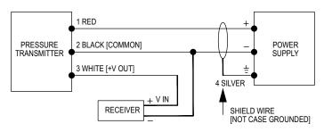
Figure E: Voltage output connection
