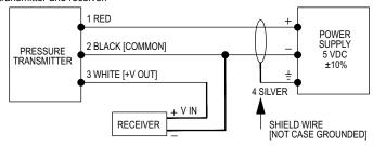
Figure K: Voltage output connection
