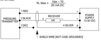
Figure A: Current output connection
