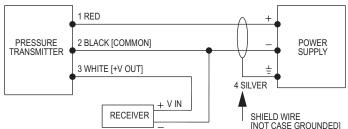
Figure D: Voltage output connection
