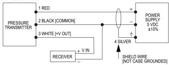
Figure G: Voltage output connection
