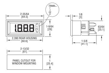
The DPMP-5 LCD Digital Panel Meter provides easy viewing on the 3-1/2 digit display. The display segments are available in a choice of amber, green or red. The meter features user selectable engineering units, adjustable zero and span, and field selectable decimal point position. The snap-in bezel mount eliminates mounting hardware.
