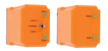
**The Series DPC** is used in control panels where two loads are required to alternate to provide equal run time on the loads. The alternating action is initiated by a control switch, which is common with one side of the control voltage. The output contacts will change states each time the control switch is opened, thus alternating the two loads. The LED indicators show the position of the output relay.
