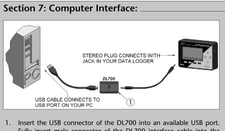
Fully insert male connector of the DL700 interface cable into the female receptacle of the data logger\*.
