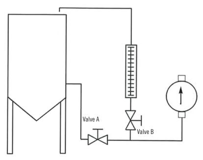
Install the calibration column on the inlet side of the pump to be checked. The calibration column must be mounted in a vertical position and must be below the level of the liquid in the tank so that it will fill when valves A & B are opened.
