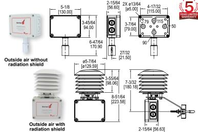
The Series BTT Temperature Transmitters offer transmitter output signals with the same form and fit as our popular TE thermistor and RTD sensors for building HVAC applications. Thermowells are required when using immersion models in liquid applications.
