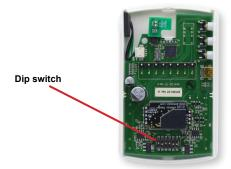
Figure 2: Diagram of circuit board
