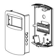
Figure 1: Removal of cover from back plate
