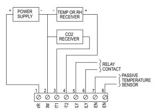
Figure 4: Active output wiring diagram
