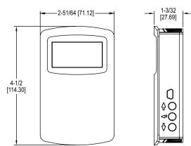
Series CDT and CDTR Wall Mount Carbon Dioxide Temperature Transmitters accurately monitor the CO<sub>2</sub> concentration and temperature in schools, office buildings, and other indoor environments to help achieve LEED® certification. Additionally, the Series CDTR also measures ambient relative humidity. In order to achieve a higher level of accuracy, the Series CDT includes digital barometric pressure adjustment.
