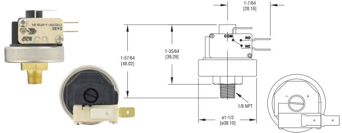
Series A9 Pressure Switches are designed for controlling pressure with higher current capacity. These switches are used widely in steam cleaners, steam irons, and other pressure control systems. It provides SPDT contact and Series A9 Pressure Switches utilize high-quality miniature snap-action switches. The switch is diaphragm operated, boasting a high temperature rating and compact size.
